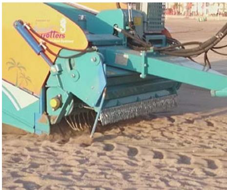
Working width of 1.9 or 2.5m depending on the version of the machine.
