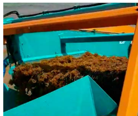
Its screening is reinforced to properly split the seaweed from the sand and get it back to the beach
