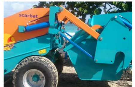
Pistons to lift and turn the hopper
