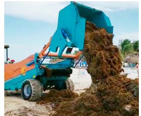
Unloading the hopper
