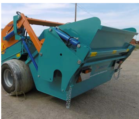
Its big size hopper allows to keep a large amount of sargassum before emptying it.
