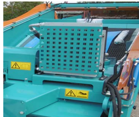
The refrigerating device allows to control the temperature of the hydraulic system.
